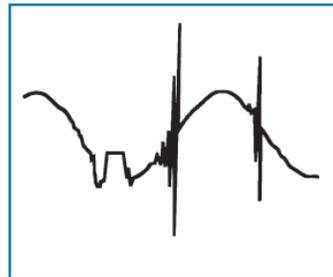
Typical Voltage Impulse Waveform
