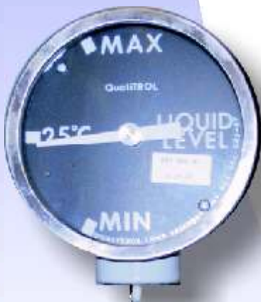
Oil level gauge
