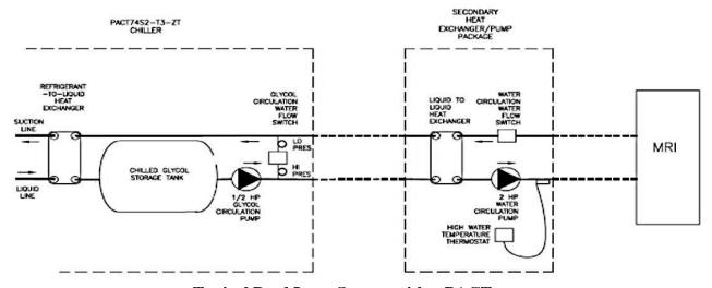
Typical Dual Loop System with a PACT Package Chiller System.
