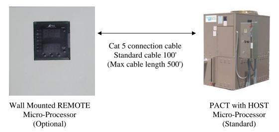
**General Description:** The Legacy remote micro-processor is a self powered device. This device make remote operation of the chiller possible from up to 500 feet away. Interface is password protected with the same review and user functions available at the host chiller's interface. This device is ideal for projects sites where adverse weather conditions can interfere with set-point changes needing to be made.
