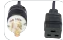
010-9338: NEMA L5-15P to C19 125V, 15A twist-lock 8-foot, 14 AWG/3-wire
