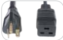
010-9337: NEMA 6-20P to C19 250V, 20A straight blade 8-foot, 12 AWG/3-wire
