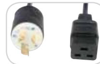
010-9340: NEMA L6-15P C19 to 250V, 15A twist-lock 8-foot, 14 AWG/3-wire
